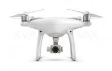
Fig. 1 Quadcopter "Phantom 4 Pro" with thermal imager "Flir-Boson"
