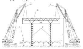
Figure 1 – Installation of the structural block of a covering by the crane way
