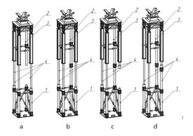
Figure 4 – PfP lifting sequence (grease frame conditionally not shown):  $1 - mounted \ tier \ of \ the \ column;$  2 - PfP;
