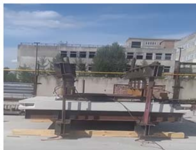
Figure 8. A fragment of an experimental study of a reinforced concrete wall
