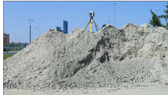
Figure 6: Scanning of the piles at the Apollo bridge in Bratislava
