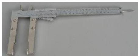
Picture 2: Sliding calliper to measure width dimensions (source: URL: < http://www.fsp.s.muni.cz/laborator >)
