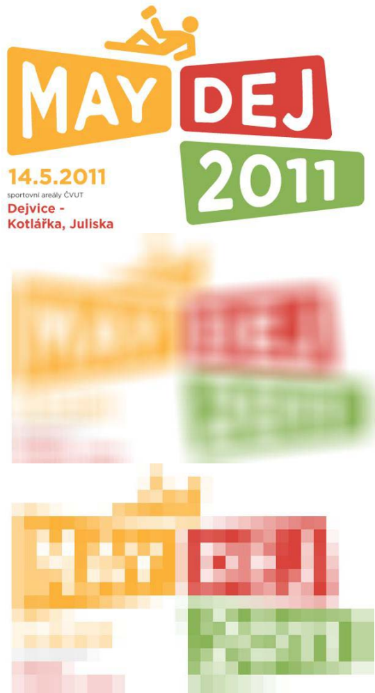
Figure 5 –Comparison of low-pass filtering (center) and the mosaic approach (below) applied to a test image (above).
