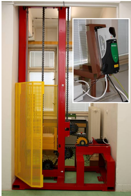
Fig. 1 Experimental station for dynamic tests of gearings with members of the management (The real view)
