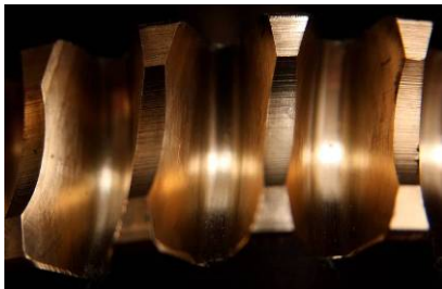
Fig. 7 The tooth flanks surface of unused gearbox worm wheel.
