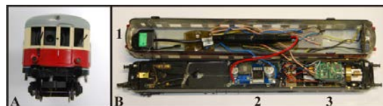
Figure 7: Integrated camera: A) front view, B1) side view, B2) DC/DC converter, B3) microcontroller
