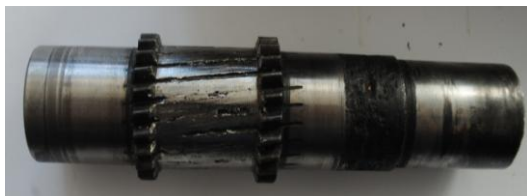
Figure 2. The pinion damage.
