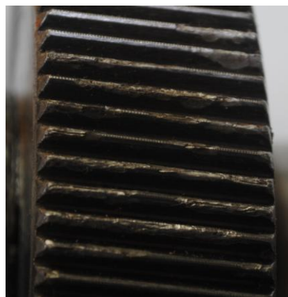
Figure 4. Damage to the teeth of gear wheel.
