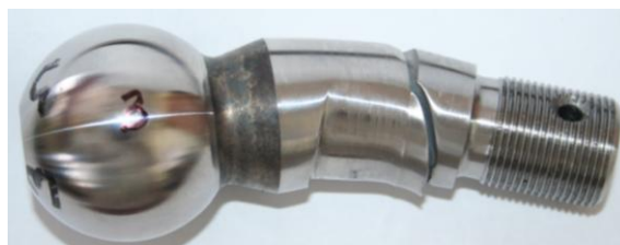
Figure 8. The appearance of the destroyed parts made of steel 40X.
