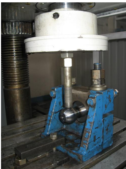
Figure 6. The scheme of fastening and loading of ball fingers during bench tests.
