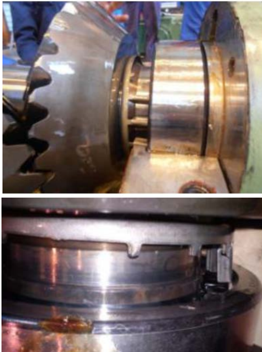
Figure 2. Damaged bearing on input shaft.
