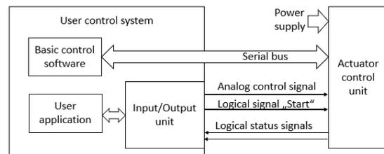
Figure 9 Block diagram of the control
