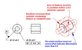
Figure 9. Example of position tolerance.
