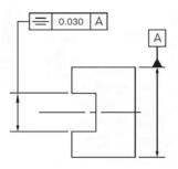
Figure 10. Example of symmetry tolerance.
