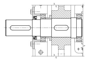
Figure 12. Part of the assembly drawing - input shaft positioning in bearings.
