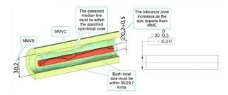
Figure 5. Combination of straightness tolerance and material maximum.
