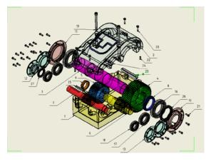
Figure 1. Elements of the gearbox.
