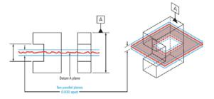
Figure 11. Symmetry tolerance zone.
