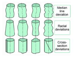
Figure 7. Deviations from the cylindrical shape.
