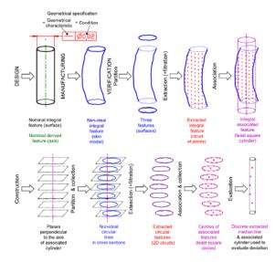
Figure 3. Definition of the basic idea of geometric dimensioning.
