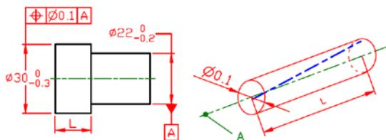
Figure 8. Example of position tolerance.
