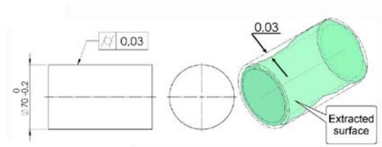
Figure 6. Example of a roundness tolerance rule at the cylindrical shaft end.
