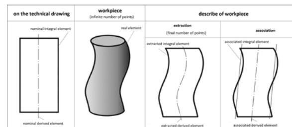
Figure 2. Definitions of geometric elements.
