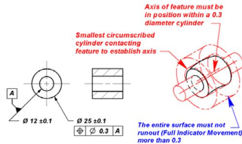
Figure 9. Example of position tolerance.
