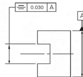
Figure 10. Example of symmetry tolerance.
