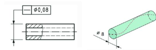
Figure 4. Straightness tolerance.
