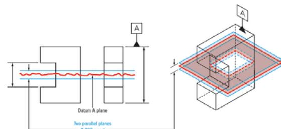
Figure 11. Symmetry tolerance zone.
