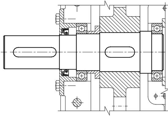
Figure 12. Part of the assembly drawing - input shaft positioning in bearings.
