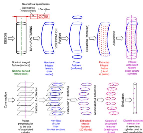
Figure 3. Definition of the basic idea of geometric dimensioning.
