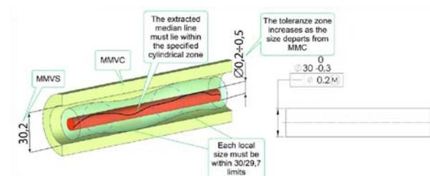
Figure 5. Combination of straightness tolerance and material maximum.
