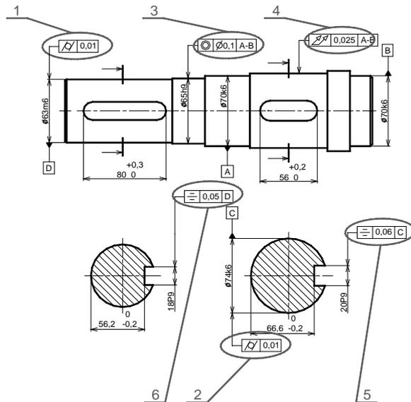
Figure 13. Prescription of geometric tolerances on the shaft – example
