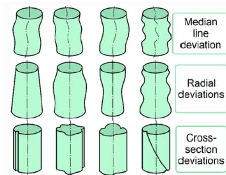
Figure 7. Deviations from the cylindrical shape.
