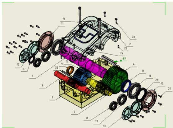
Figure 1. Elements of the gearbox.
