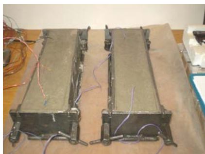
Fig. 3 Two concrete specimens intended for the temperature measurement, immediately after having been poured into the beams.
