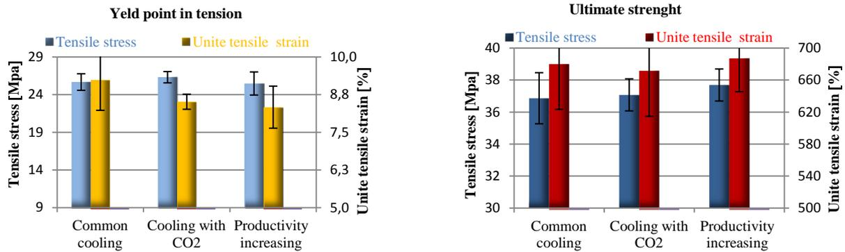
Fig. 4 Results of tensile test for PP-Mosten EH 0.1
