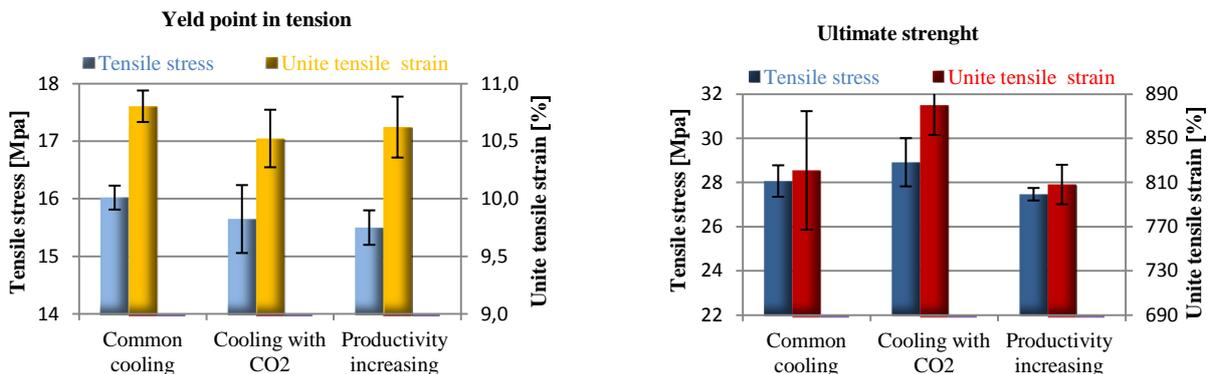
Fig. 5 Results of tensile test for PE-Liten BB29
