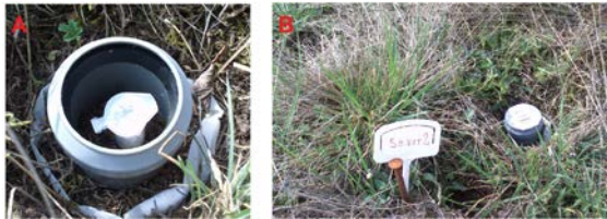
Fig. 3 Application of measuring probes with soda lime granules at experimental site Havraniky (author: Elbl).
