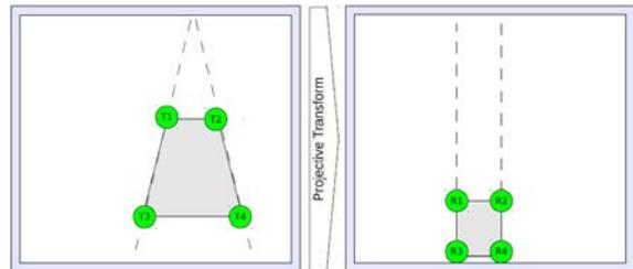
Figure 3: Projective transform mapping the corners of the cabin view to the corners of the rectangle of the bird's-eye view.
