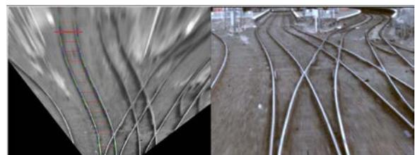
Figure 4: Transform of the image with rail tracks.
