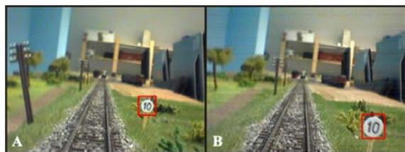
Figure 8: Sign detection: A) good quality image, B) image with noise
