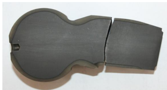
Figure 4. The contour of the layer of a part made of steel 40X hardened by high-frequency hardening.
