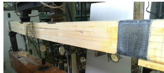
Figure 3 – General view of the reinforced beam under load
