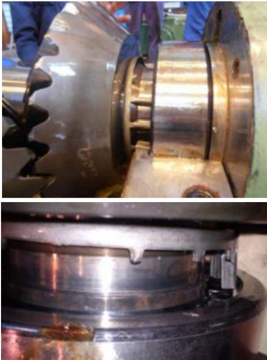
Figure 2. Damaged bearing on input shaft.
