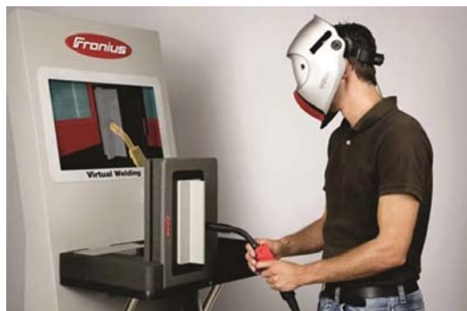
Figure 2: Welding simulator by Fronius (Source: https://www.mmspektrum.com/clanek/virtualni-svarovani-simulatory-pro-vyuku )
