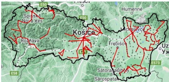
Figure 4 Bus routes identified for replacement by DRT with estimated savings over 2000€ a year
